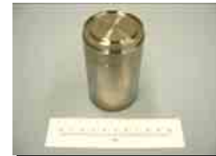
Curium capsule located at REDC – Curium is used to fabricate targets that are irradiated in HFIR for isotope production
