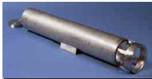
Mark 42 target located at REDC – the targets are the source of heavy elements used for research and isotope production
