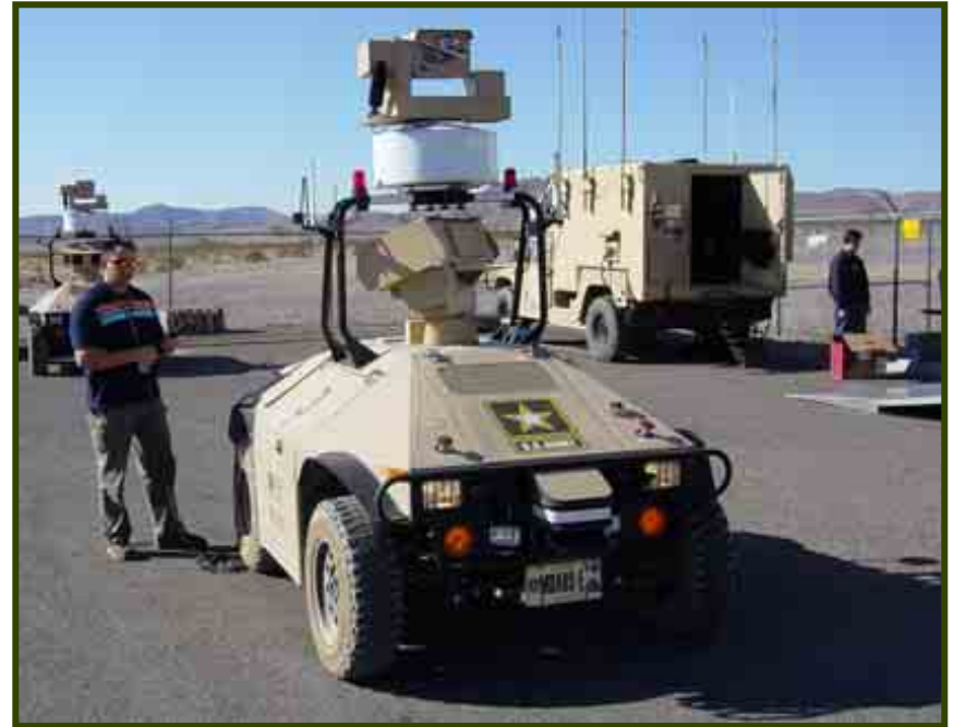
MDARS (Mobile Detection and Reconnaissance System) will be deployed at the Area 5 Radioactive Waste Management Site to enhance security
