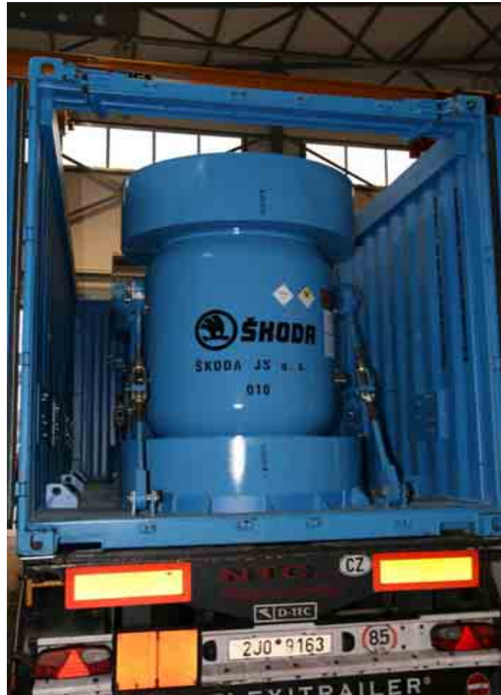
ŠKODA VPVR/M cask in ISO container
