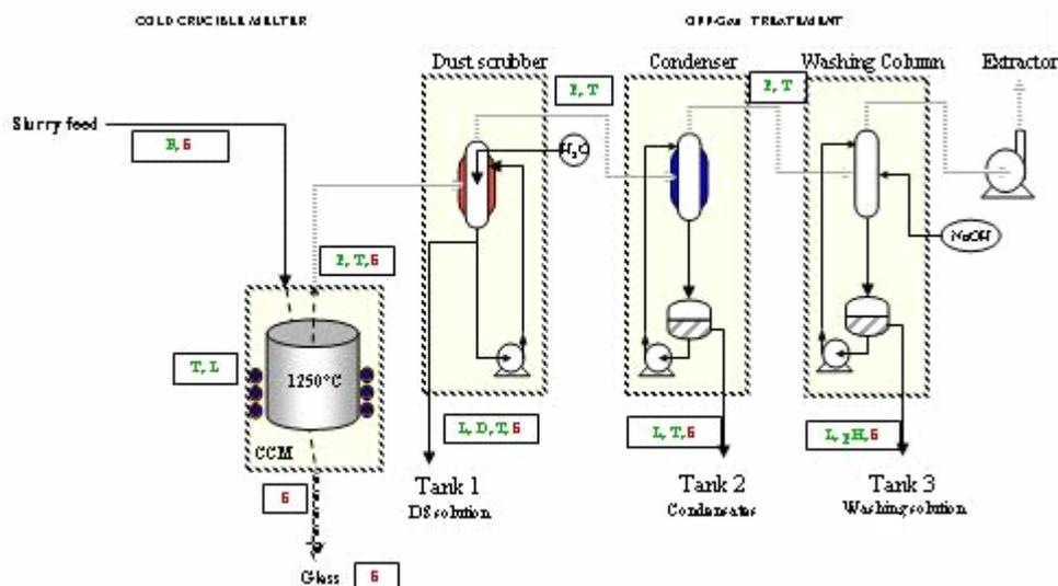
**Fig. 2. Diagram of the off-gas treatment system – CCIM platform – CEA Marcoule.**
