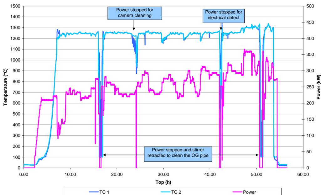
**Fig. 4. Evolution of power and temperature in the melt during demonstration run.**
