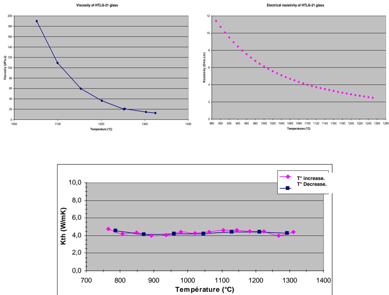
Fig. 3. Viscosity, electrical resistivity, thermal conductivity as a function of temperature – Nominal HTLG-21 glass
