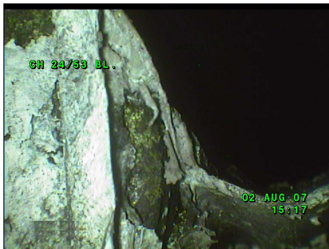
Figure 3—Partially melted fuel cartridge with fuel pin exposed.
