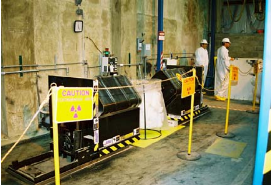
Fig. 2. Drums are loaded in “upenders” in the processing area of the Drum Cell.
