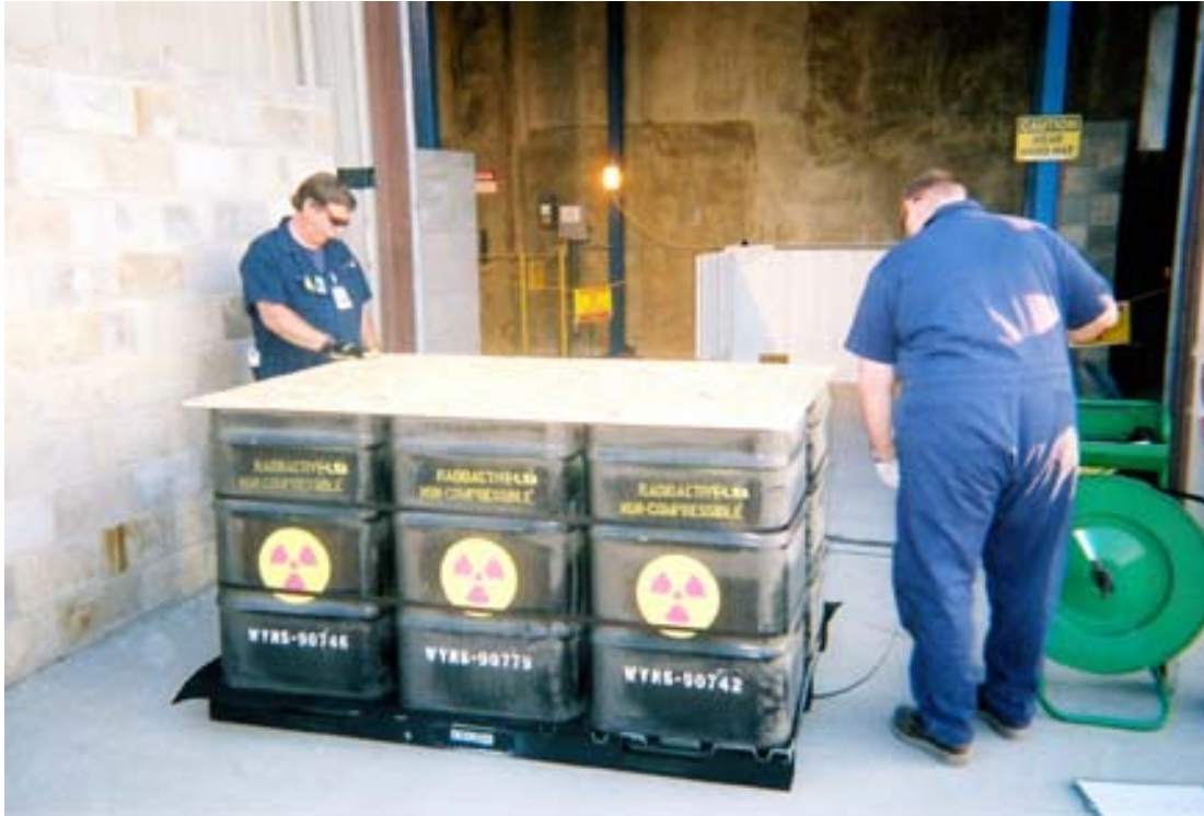
Fig. 3. Operators secure a plywood top to a pallet load of six drums in preparation for shipment.
