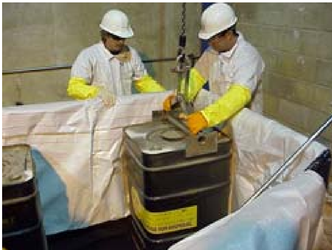
Fig. 4. Operators lower a drum into an IP-2 bag.
