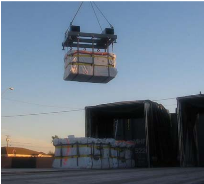
Fig. 8. Drum packages are off loaded at the Parker, AZ transload facility.
