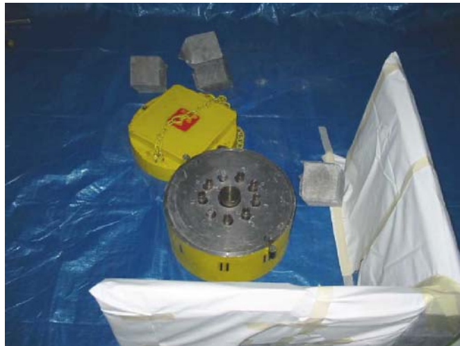
Figure 1. A loaded shielding device (the sources are inside the protruding capsules).
