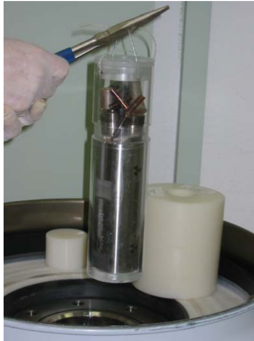
Figure 4. Transuranic sources conditioned in a certified package.
