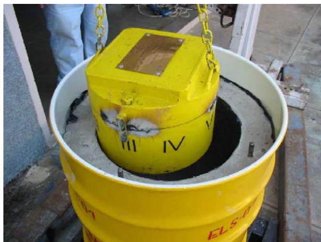
Figure 2. A locked and labeled lead shield being inserted into the shielded 200L drum.
