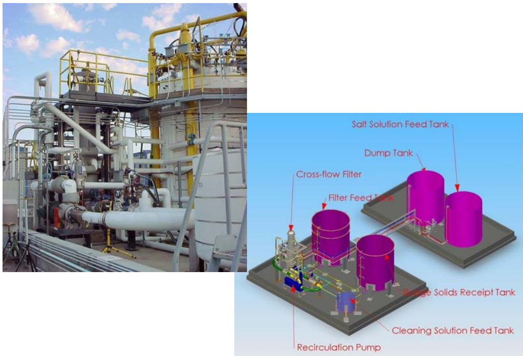
Fig. 1. Overall layout of CFF test system
