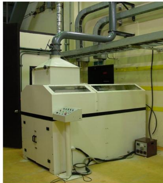
(b) Shaping compactor
