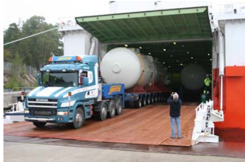
Figure 7 and 8: LOADING of the Steam Generators onto the transport ship and unloading in Sweden
