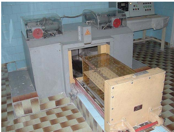
Fig 2. Cs-137 irradiator used for research purposes (before dismantling).
