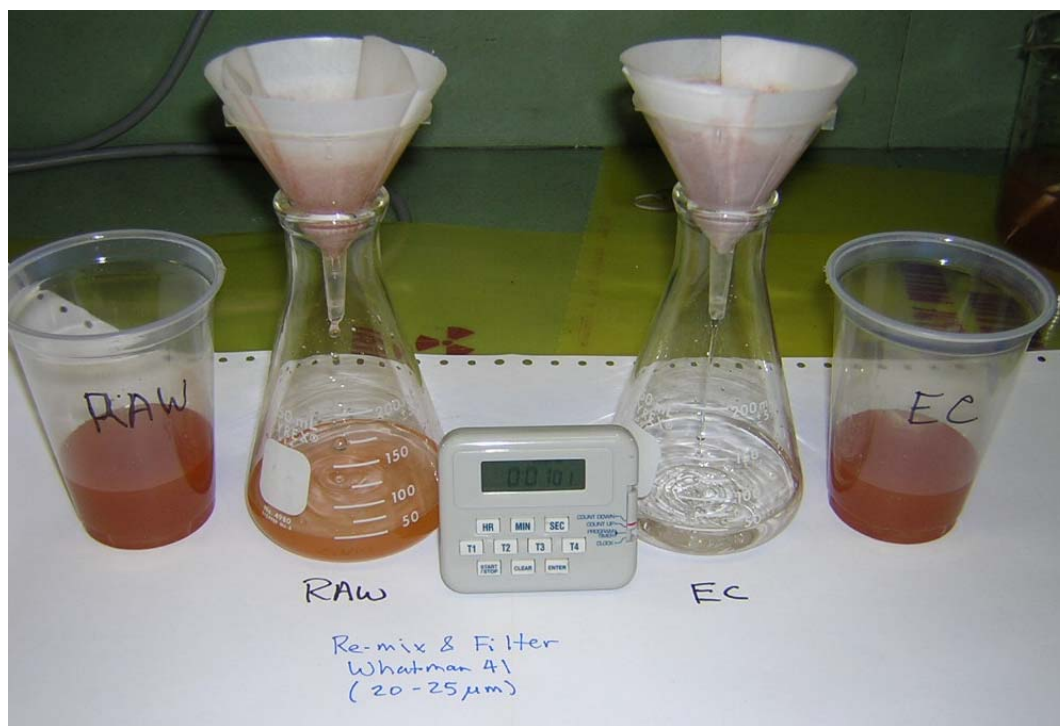
Figure 12. Filtration of raw sample (left, filter plugged) and EC-treated sample (right). Both samples were mixed well before filtration with Whatman 41 paper (nominal retention of particles > 20- to 25- \mu\text{m} , which emulates standard sheet filters).
