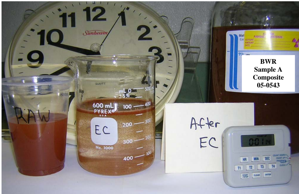
Figure 10. Sample EC (right) represents electro-coagulation for ~ 1 amp-min, followed by ~ 1-min quiescent settling.
