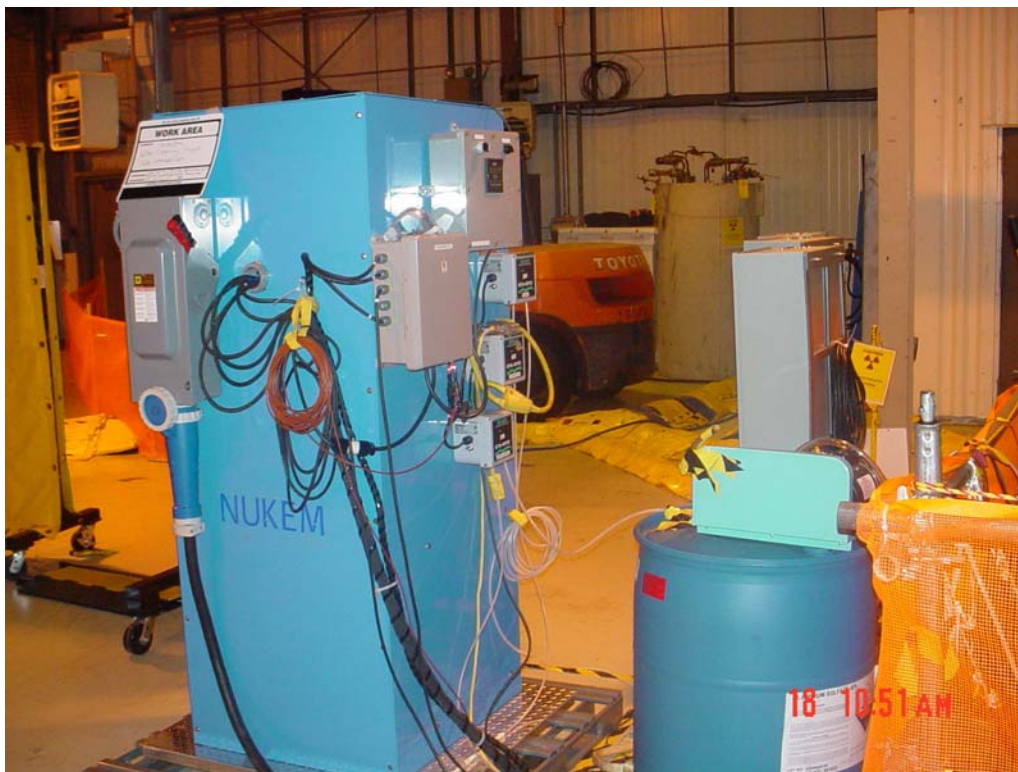
Figure 4. Chem-Add System with alum addition drum and control panel mounted feed pumps
