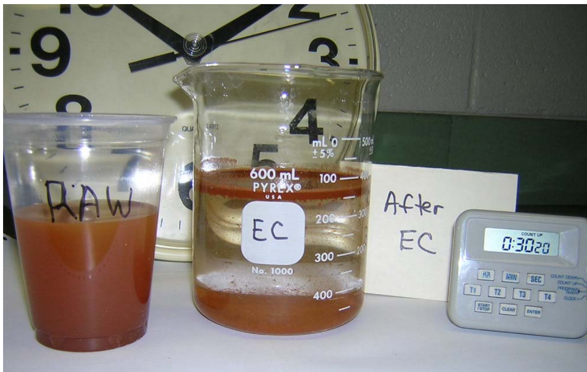
Figure 11. Sample EC (right) represents electro-coagulation for ~ 1 amp-min, followed by ~ 30-min quiescent settling. The untreated sample (left) shows minimal settling during this time interval.
