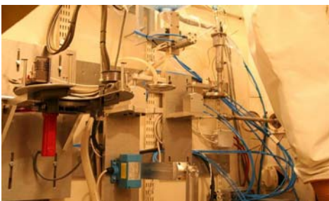
Picture 6: Workbench setup for Beryllium conditioning in Hot Cell
