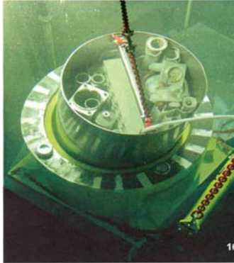
Picture 3: GNS-Mosaik container, under-water loading
