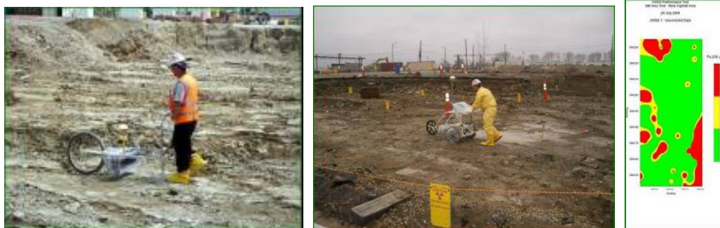
Figure 4. AXISS performing survey and a contour plot of Building-38 survey performed by the AXISS at the MCP in 2004.
