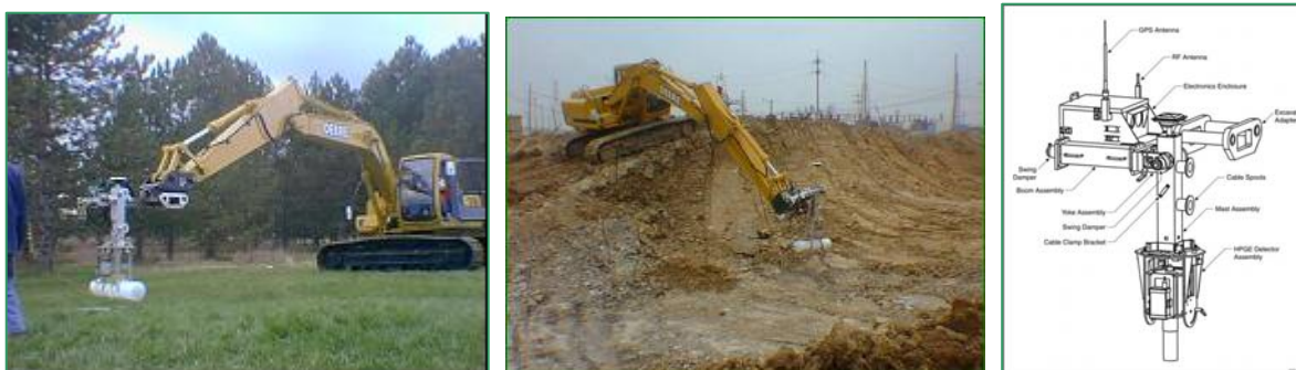
Figure 3. EMS NaI platform is used to survey trenches.
