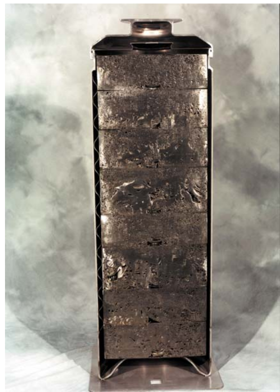
Figure 3: Compacted Discs in the CSD-C canister
