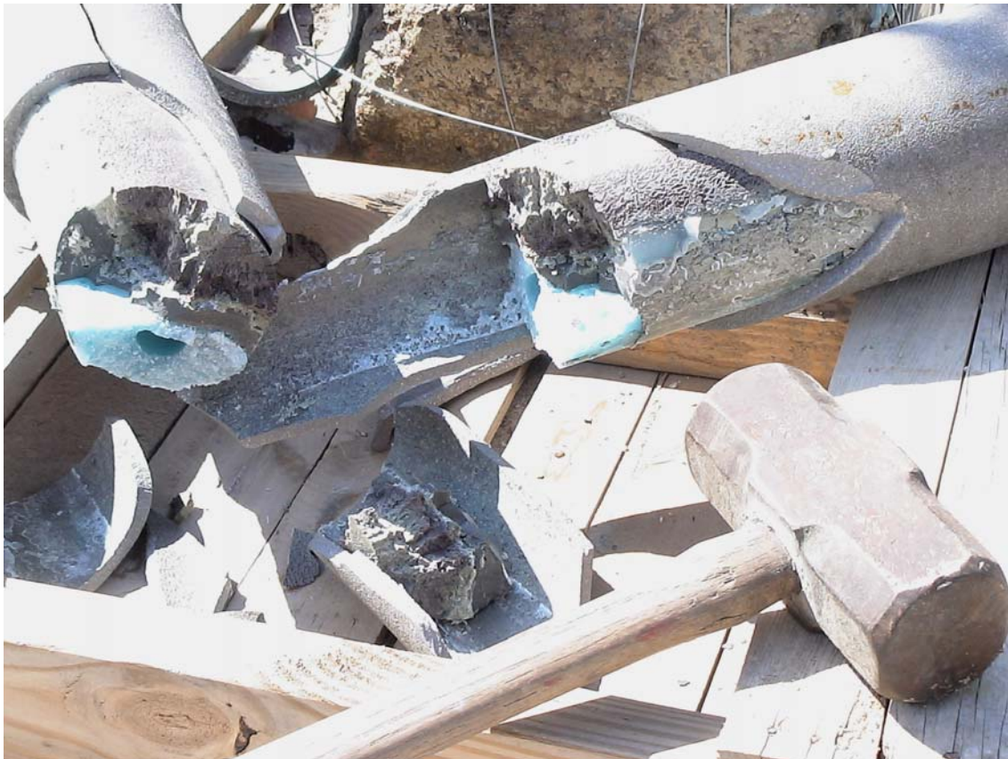
Fig. 4. Pipe 1, Dry bentonite surrogate with cement grout cap, broken with hammer
