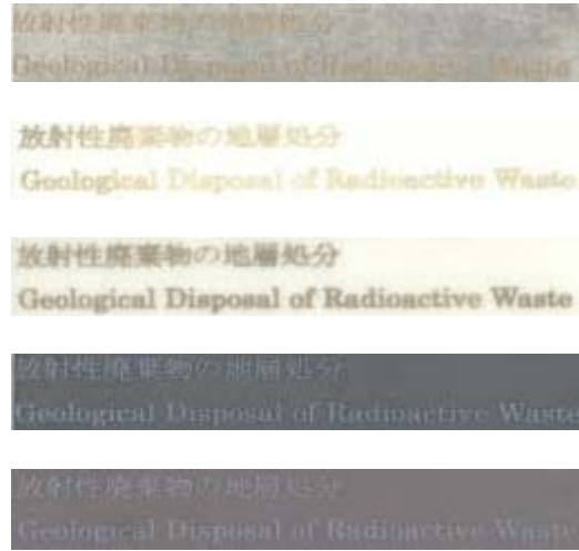
Fig. 5: Comparison of the Results of the Dot Engraving Test (From above to bottom, hastelloy, alumina, zirconia, silicon carbide sintered compact, and silicon carbide (CVD). The size of character is 11 points.)
