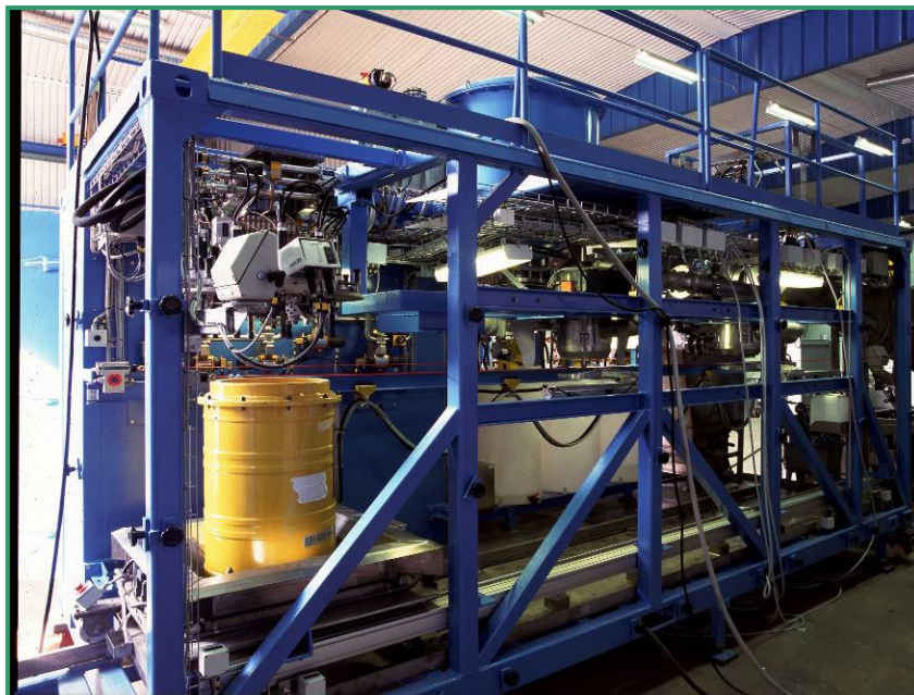
Fig.1. The MOSS waste solidification system used to cement encapsulate spent fuel sludges
