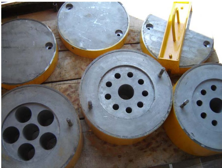
Fig.3. The packaging for long term conditioning of radium sources
