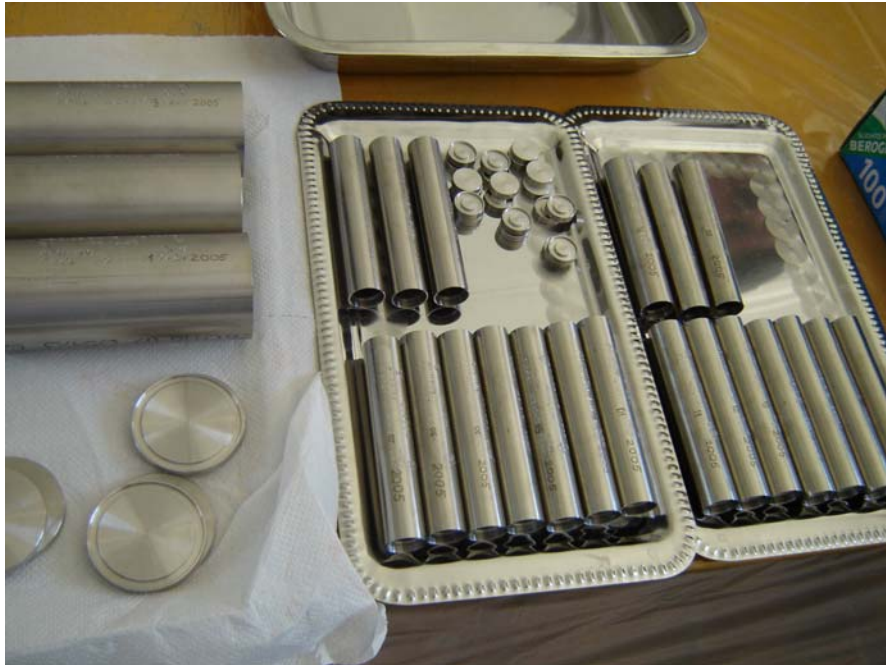
Fig. 2. The stainless steel capsule for long term conditioning of radium sources
