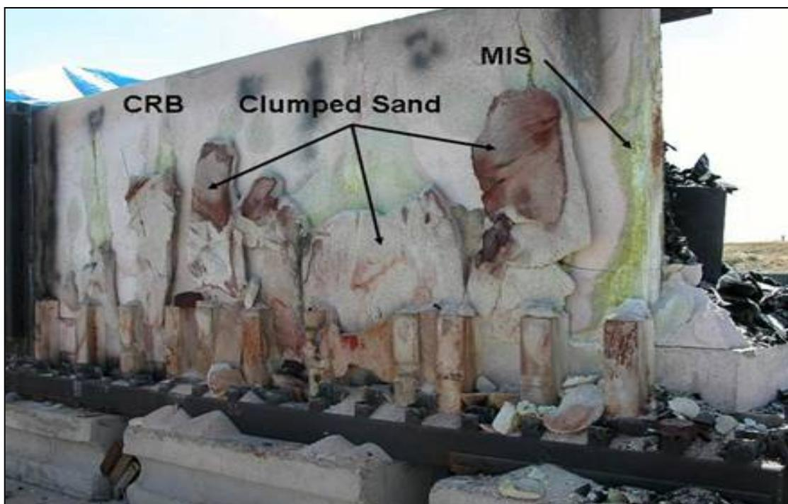
**Fig. 1 Full Scale Test 38C Refractory with MIS Deposits**
