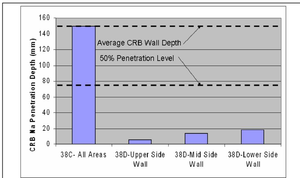
**Fig. 6 Sodium penetration depths into the CRB.**
