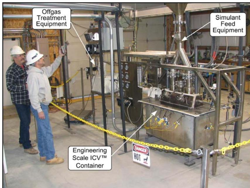
Fig. 2 GeoMelt® engineering-scale ICV™ equipment.
