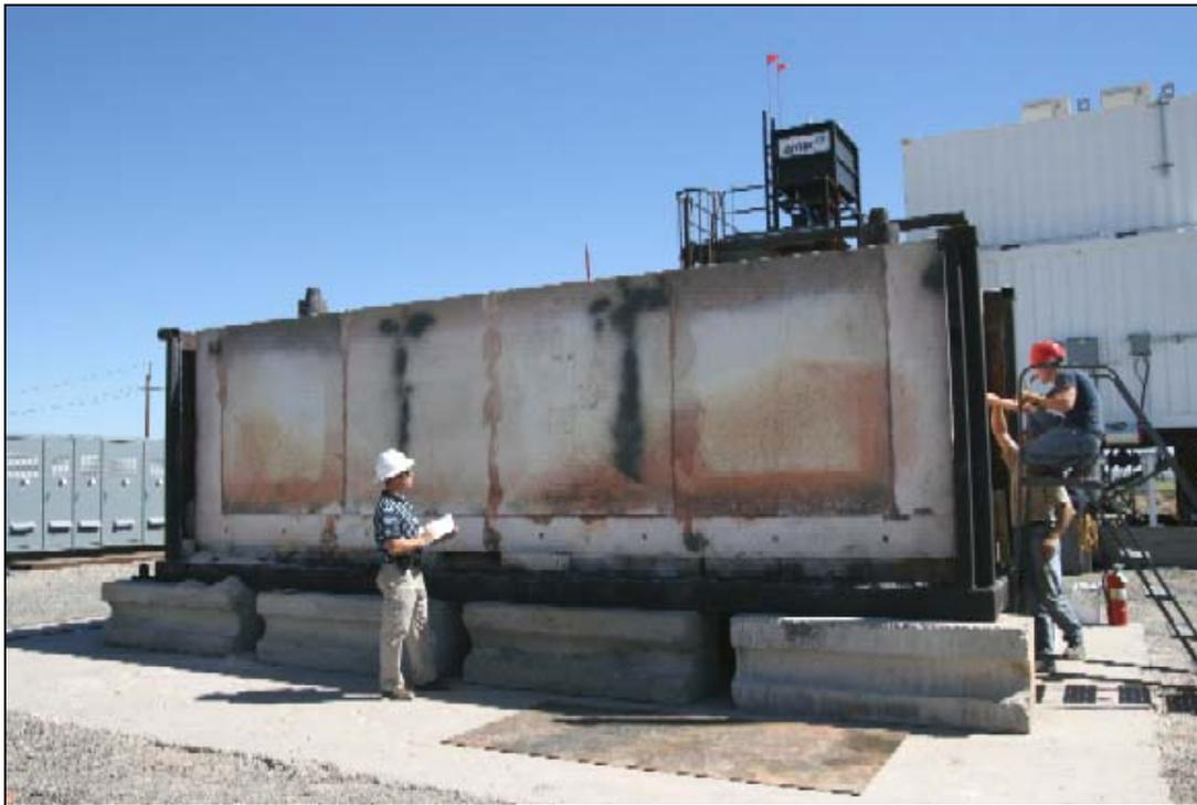
**Fig. 5 FS-38D refractory liner external skin after test completion.**
