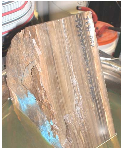
Fig. 1. Capillary wicking of wax (wet areas) upward through shale rock core sitting in pan of wax. Only the small light colored area in the upper right corner is not yet saturated.
