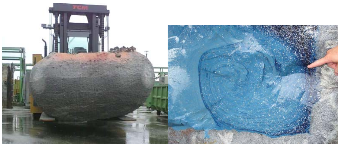
Fig. 4. Resulting glass block at left following removal from the melt container and interior of glass block at right showing convective flow patterns.
