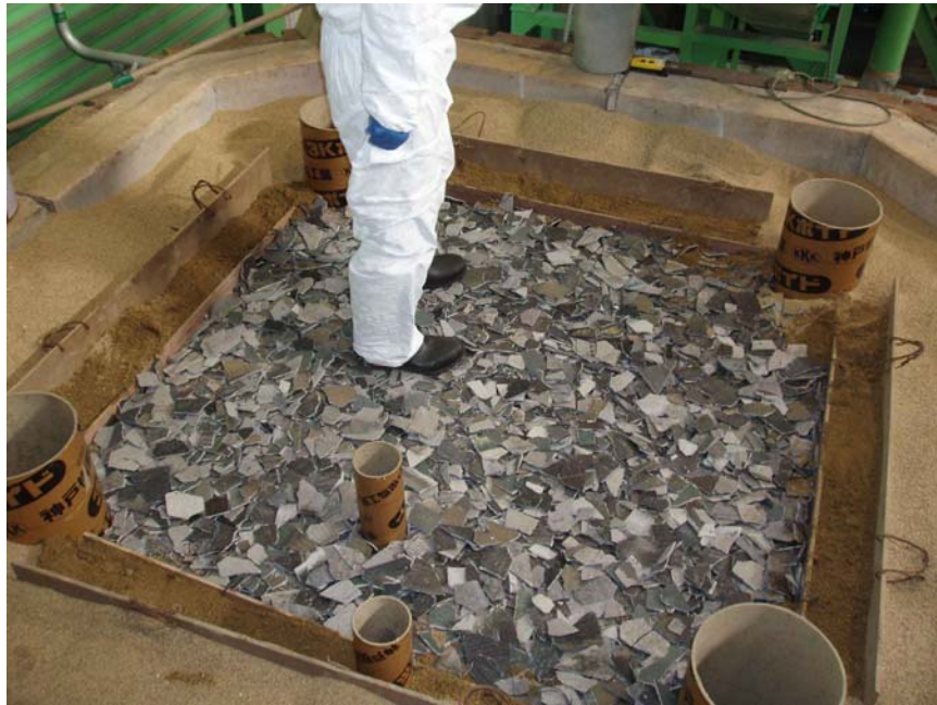
Fig. 2. View of asbestos waste material loaded into the melt container.
