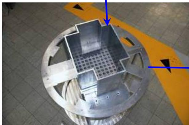
Fig. 12 Mock-up of the reactor tank internals on a 1:1 scale
