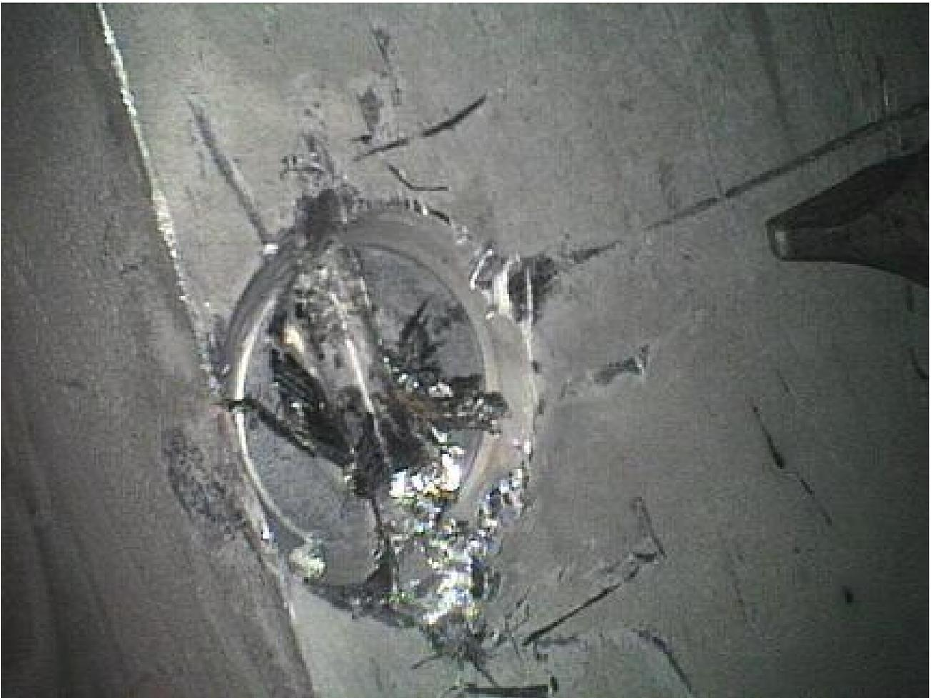
**Fig. 5. Damaged screw in the reactor tank**
