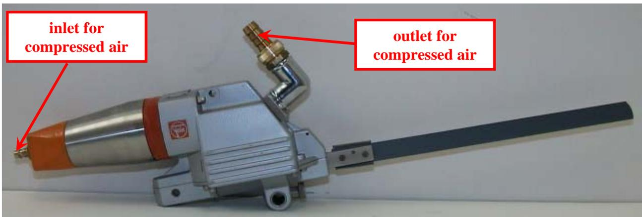
**Fig. 8. Pneumatic compass saw upgraded for underwater applications**
