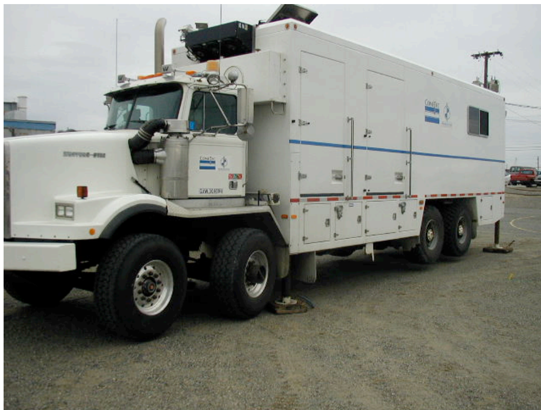
Fig. 3. 40 Ton Cone Penetrometer Direct Push Rig.
