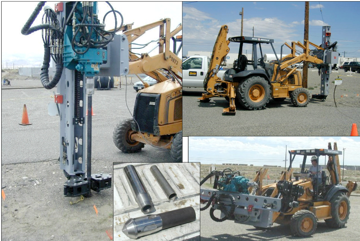
Fig. 2. Hydraulic Hammer Rig Direct Push Technology.
