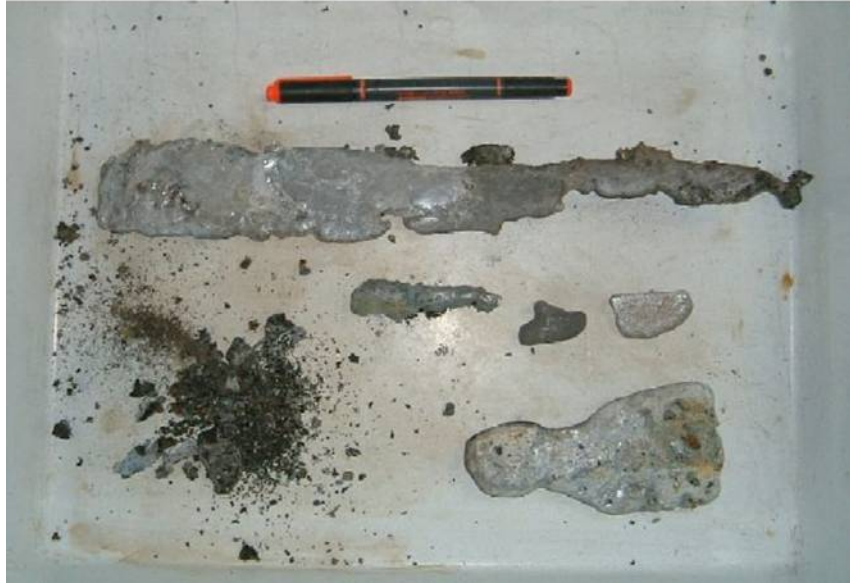
Fig. 4. Melted lead and aluminum collected in the bottom tray
