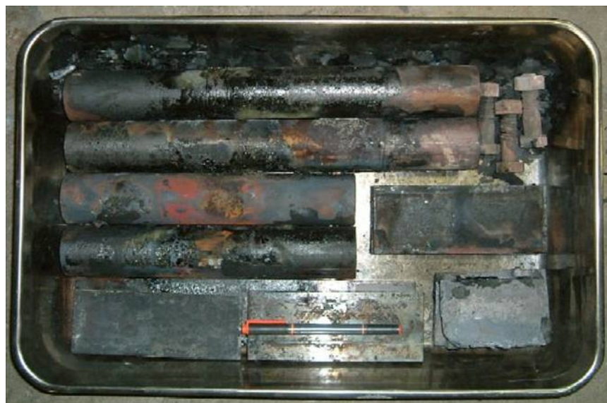
Fig. 3. Unmelted pipes and plates collected in the rotating cage
