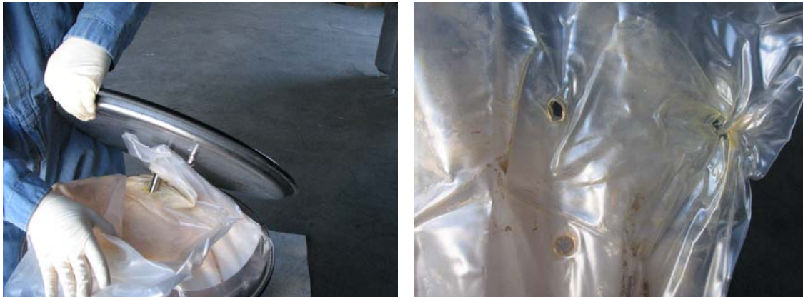
Fig. 6. (Left) Long-Stem Filter Penetration; (Right) Bag Breaching Through Multiple Layers.
