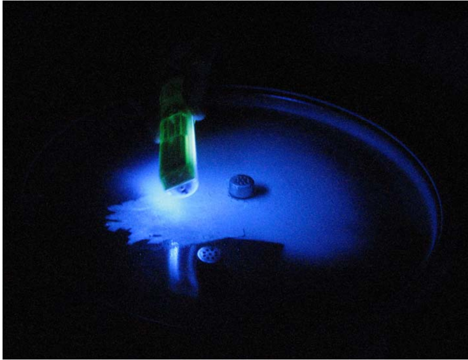
Fig. 5. Breach Bag Testing – UV Light Check.
