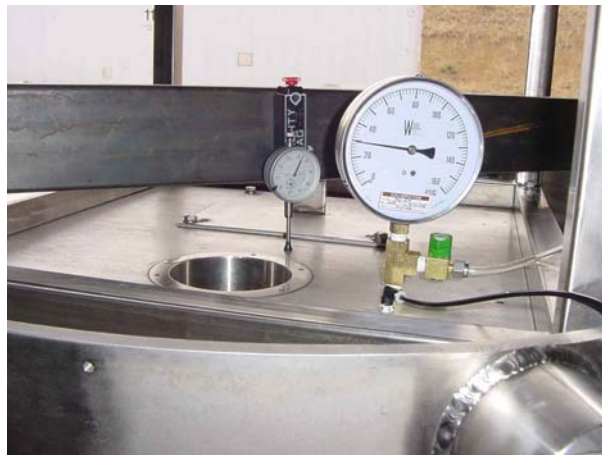
Fig. 2. Containment Chamber Test Fixture.
