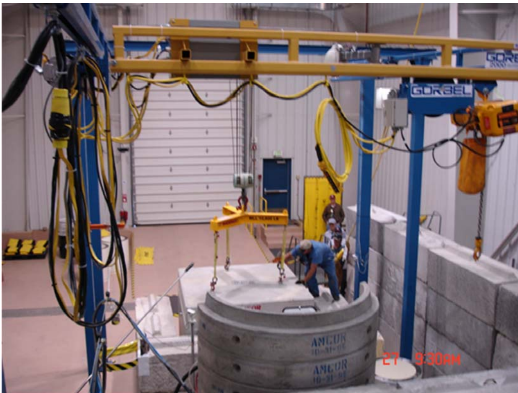
Fig. 3. Assembled RH TRU Drum Venting System.
