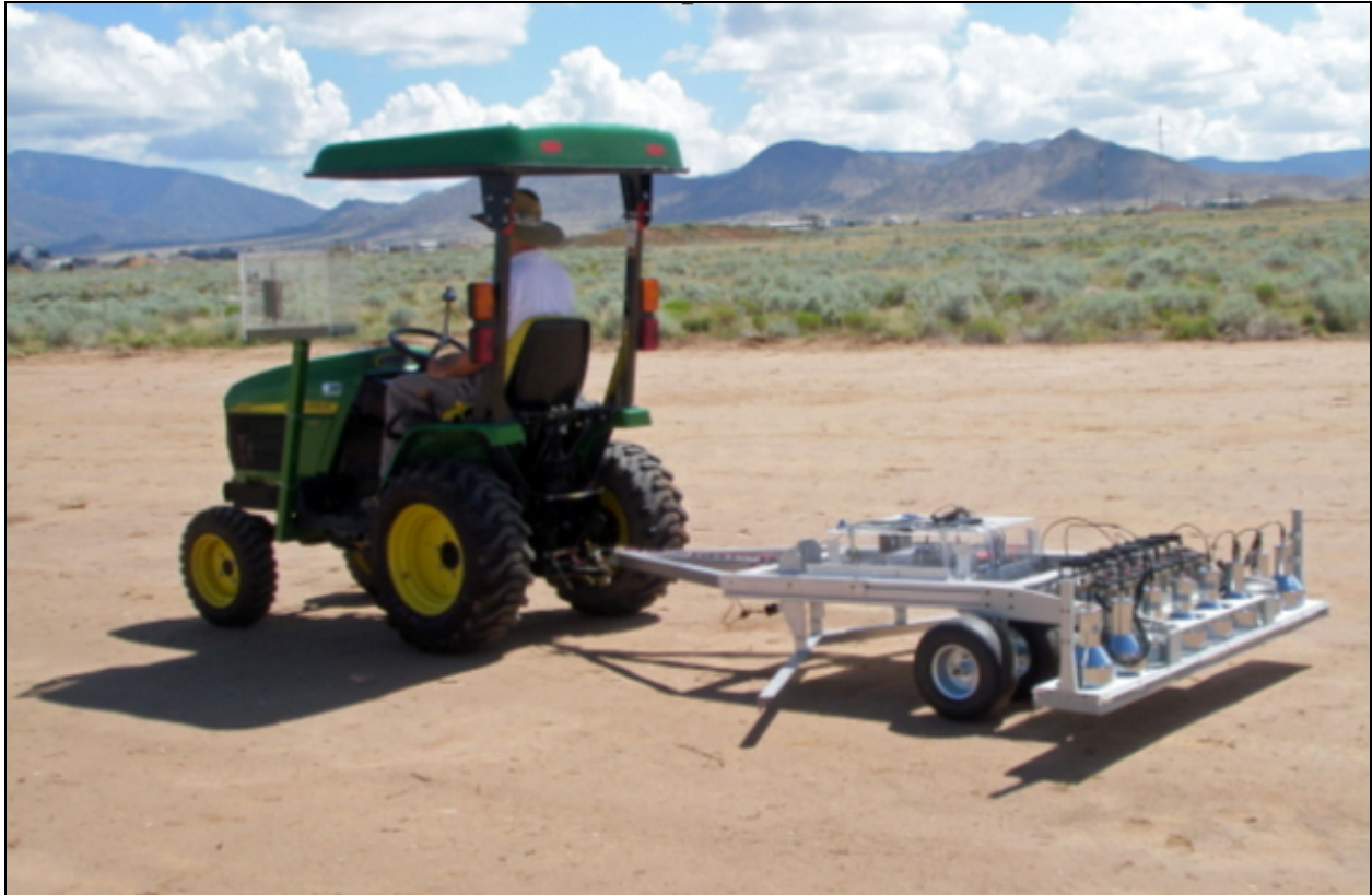
Fig. 3. Eight detector array and associated electronics pulled by tractor.
