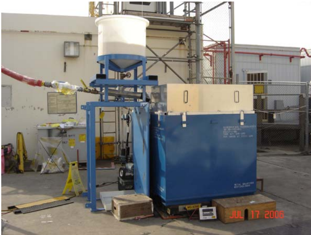
Fig. 1 Absorption of concentrates at San Onofre Nuclear Generating Station (SONGS)
