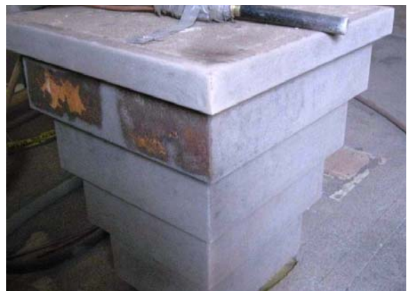
Fig. 10. Remediated plug, free released and to be used as backfill.
