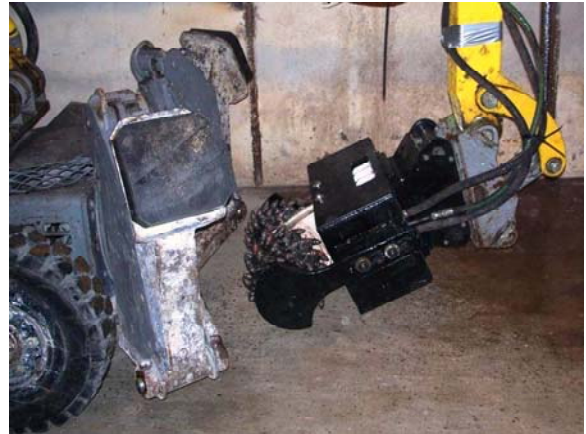
Fig. 8. Scaling drum used to remediate the floors of hot cells and the hot pipe tunnel.
