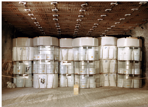
Fig. 1. Over 10,000 CH nuclear waste drums and standard waste boxes emplaced within 1 of 56 rooms to be filled at WIPP over a 20-year period. 20 rooms have been filled as of this writing.
