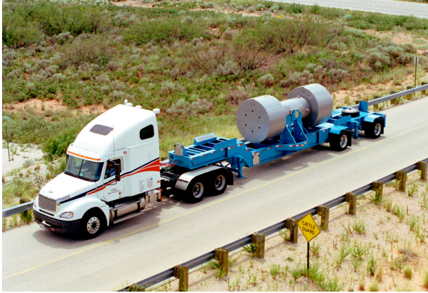
Fig. 2. Remote Handled nuclear waste (>100 nanoCi/gram of waste but <23 Ci/liter), some of it from reprocessing, being transported to the WIPP site in New Mexico in a 72B cask.
