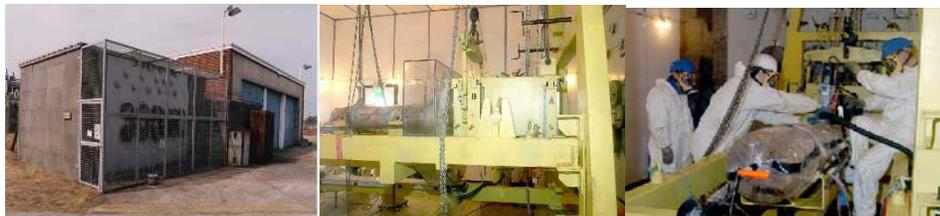
**1. Beam Plug (BP) Store    2. BP withdrawal shielding and cutting equipment    3. Assaying the LLW section of a beam plug**
