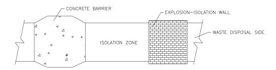
Fig. 1 Option D. Explosion Isolation Wall and Concrete Barrier with DRZ Removed
