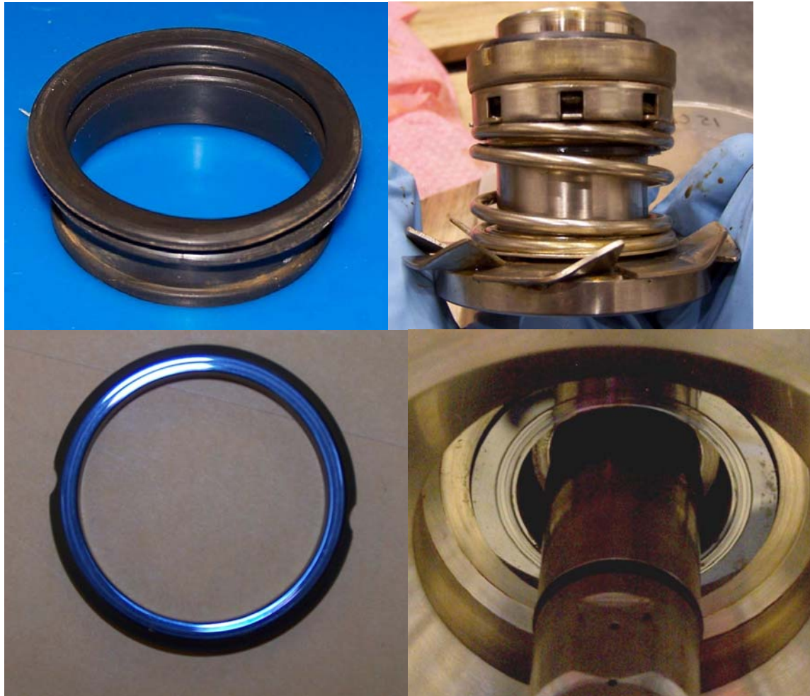
Fig. 2 The shaft seal after 120 hours of testing
