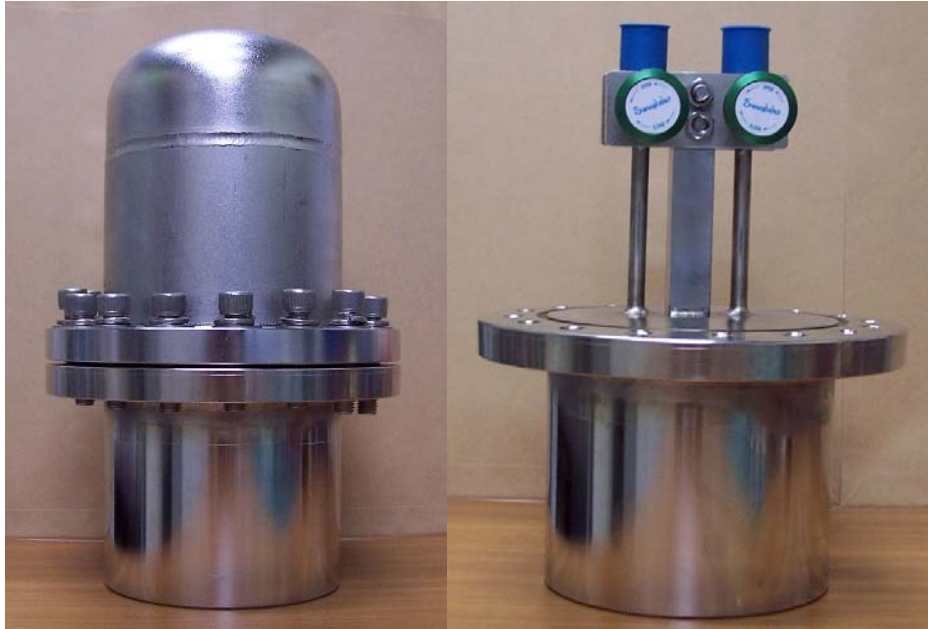
Fig. 3. Tritium storage vessel (right) with secondary container (left).
