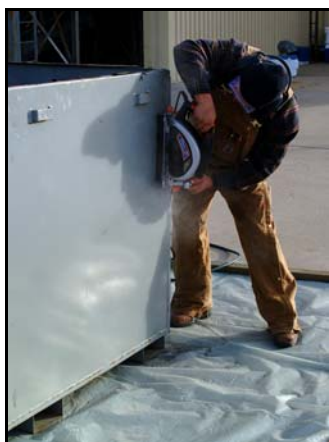
Fig 2. B-25 box being cut open.
