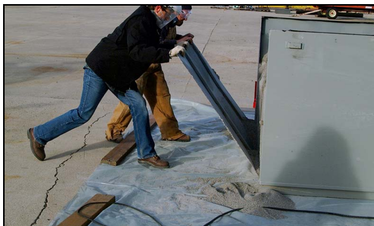
Fig 3. B-25 box being opened to check samples for void spaces and sample consistency.
