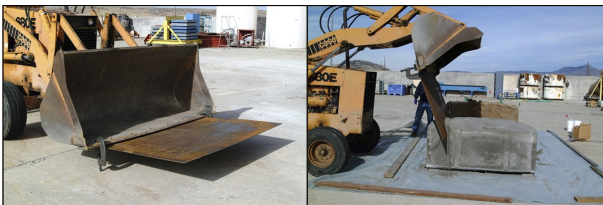
Fig. 6. Sampling tool and sampling approach for the B-25 box samples.
