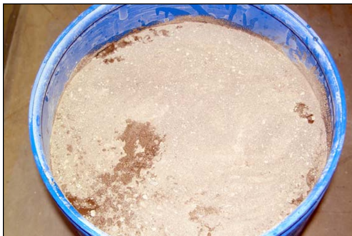
Fig. 15. Sample after Petroset II-G addition.
