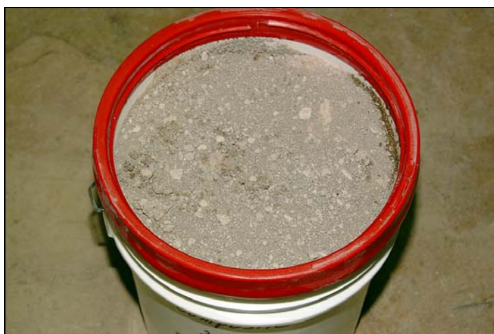
Fig. 5. Composite surrogate and Petroset II-G sample at the 2.6:1 waste-loading ratio after the 14-day curing period.
