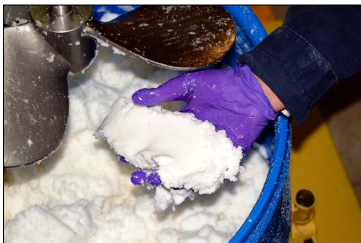
Fig. 11. Composite surrogate and Nochar sorbent sample consistency immediately after mixing.
