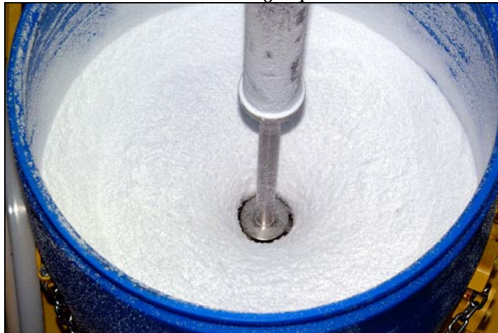
Fig. 6. Nochar sorbent being mixed prior to surrogate introduction.
