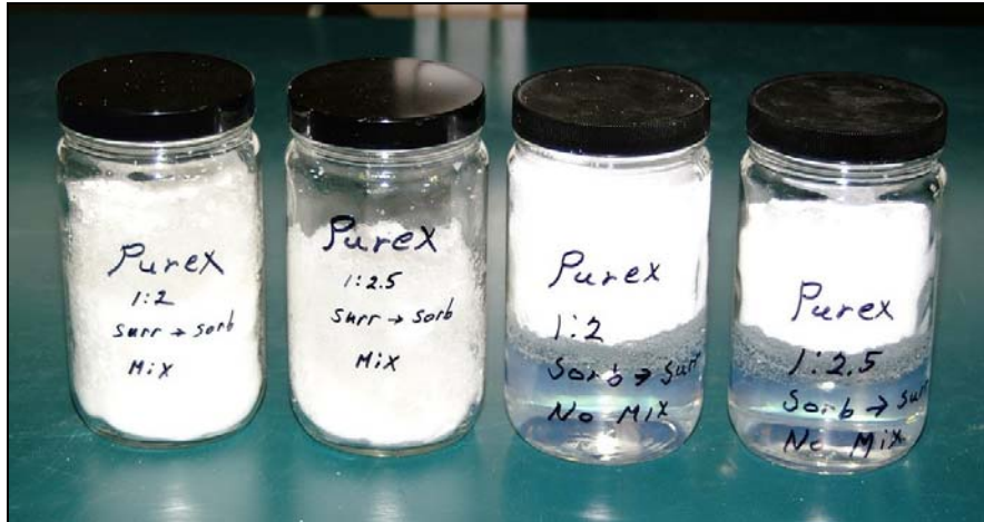
Fig. 1. Mixed and unmixed Nochar and PUREX surrogate samples.
