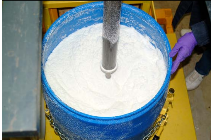
Fig. 9. Composite surrogate and Nochar sorbent during the 6-s mixing window.
