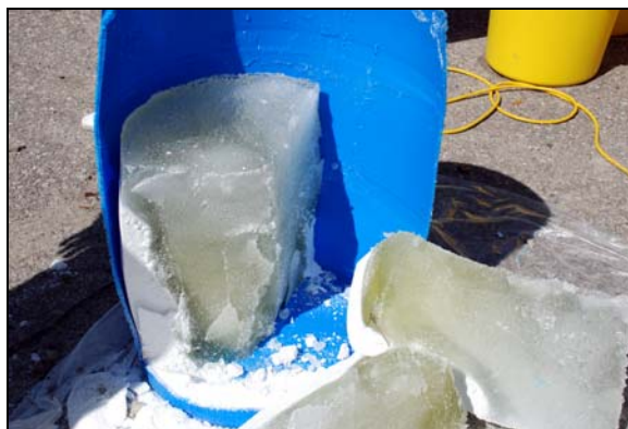
Fig. 21. Nochar sample during physical destruction of the sample.
