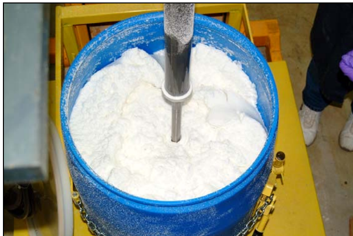
Fig. 10. Composite surrogate and Nochar sorbent after 6-s mixing window at the point where mixing stops being effective.
