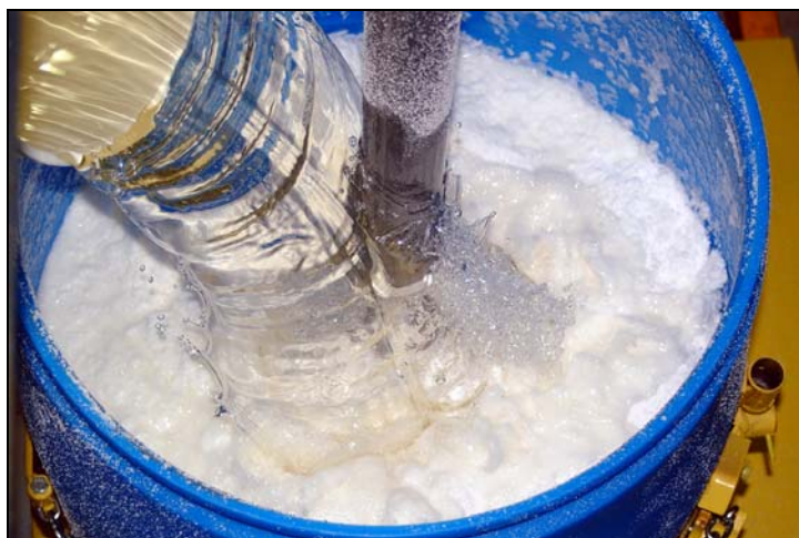
Fig. 8. Addition of composite surrogate to the Nochar sorbent while mixing.
