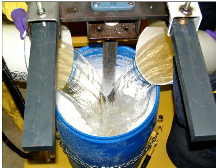
Fig. 7. Addition of composite surrogate to the Nochar sorbent while mixing.
