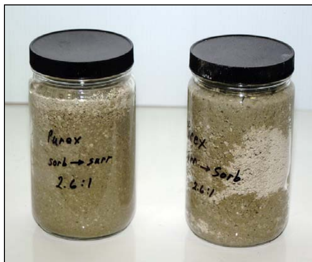
Fig. 3. Organoclay samples generated using different addition methods at the 2.6:1 ratio.
