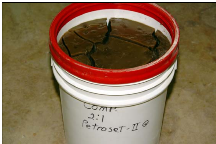
Fig. 4. Composite surrogate and Petroset II-G sample at the 2:1 waste-loading ratio after the 14-day curing period.
