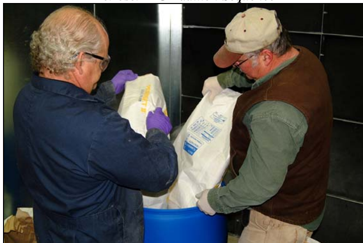
Fig. 14. Addition of Petroset II-G into the composite surrogate wastestream.
