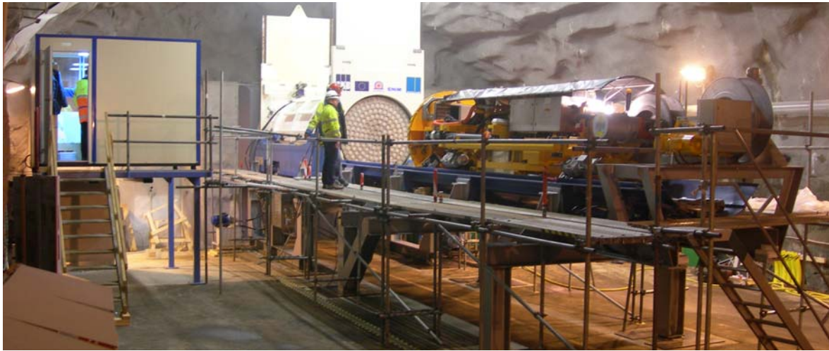
Fig. 3. Set-up of equipment at the Äspö HRL (level -220 m) test site. The SC is inside the transport tube with the shielding gamma gates open (the control room is on the left side of this photo).
