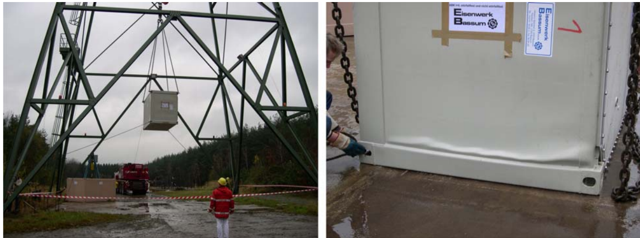
Fig. 3. Steel container KONRAD Type V drop test; ABK I+II with accident safe waste packaging; 5.0 m drop height.
