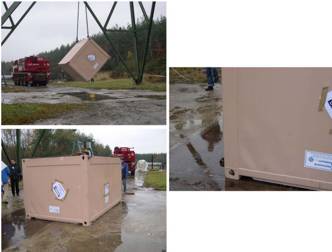
Fig. 2. Steel container KONRAD Type V drop test; ABK I; 80 cm drop height.
