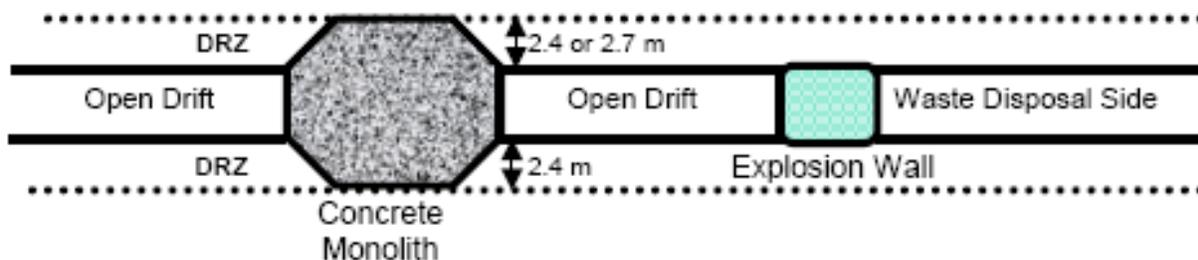
**Fig. 1. Panel Closure System (PCS) proposed by the DOE in the CCA for use in the WIPP repository.**
