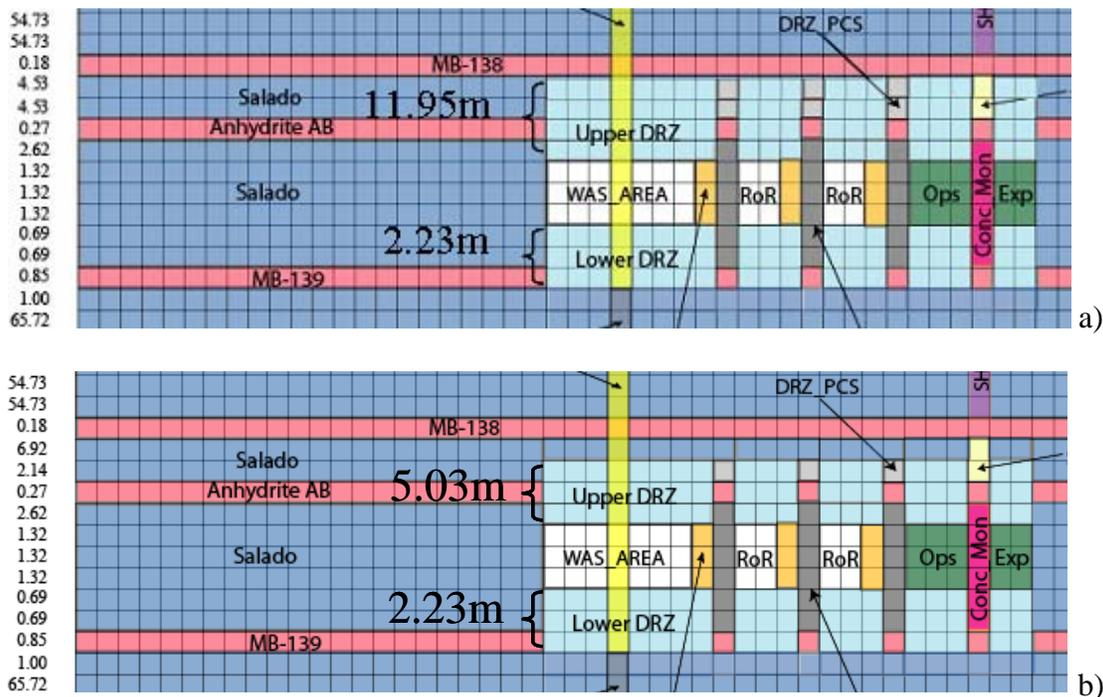
**Fig. 2. DRZ modeling for the a) CRA-2004 PABC and the b) scoping calculations, DRZ extent in the BRAGFLO grid. (Scale on left side indicates cell height in meters.)**
