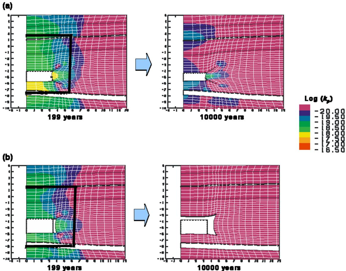
**Fig. 3. Permeability of damaged halite in the Disturbed Rock Zone (DRZ) around the WIPP repository as a function of time for the (a) minimum and (b) maximum gas generation rates. Permeability represented on a logarithmic scale. Taken from Park et al. [12].**
