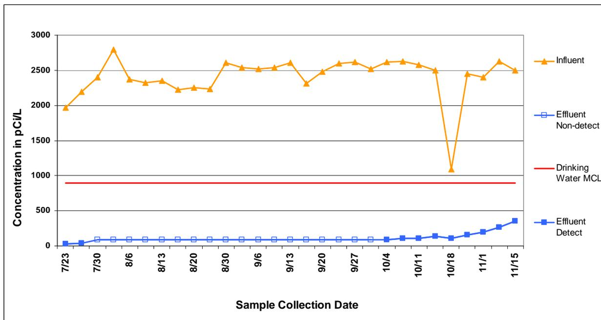
Fig. 2. Technetium-99 data is presented from the resin column on extraction well 299-W15-765.
