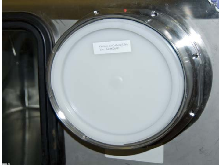
Figure 4. Gloveport Plug Configuration.
