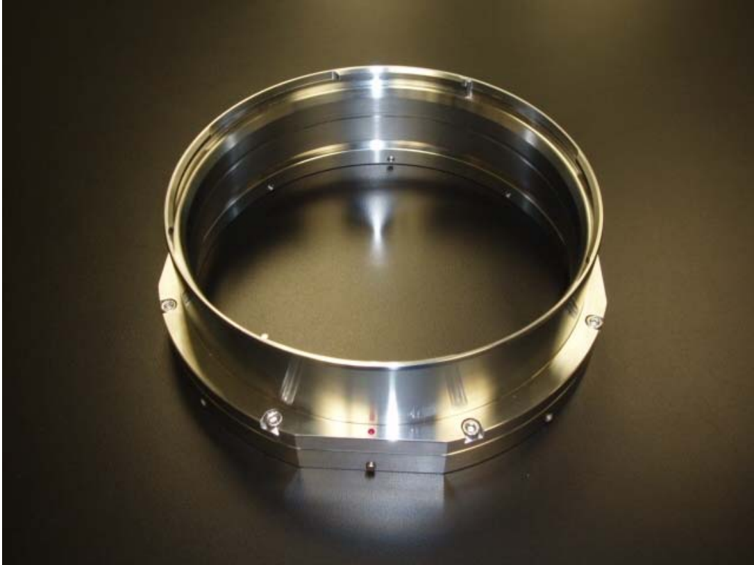
Figure 3. Assembled Gloveport Retrofit. 1
