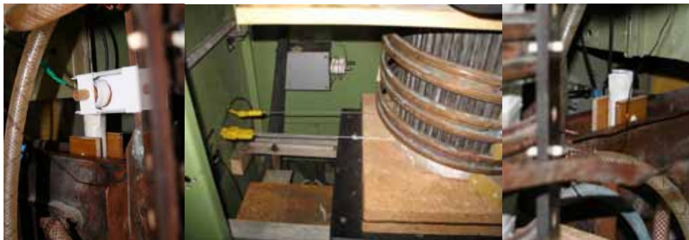
Figure 2 - Configuration and location of phase angle (current component), voltage, and current sensors, respectively, on the ETU LETI Test Melter
