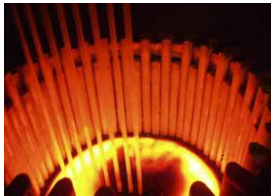
Figure 4 - Deployment of High Temperature Thermocouples in the Test Melter at ETU LETI
