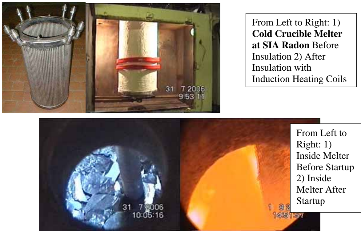
Figure 1 – Increasing Nuclear Waste Loading in DOE High Level Waste Glass Using a Cold Crucible Induction Melter
