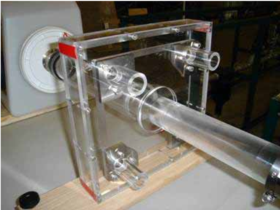
Figure 4 - Demonstration model VXA fitted to Glovebox
