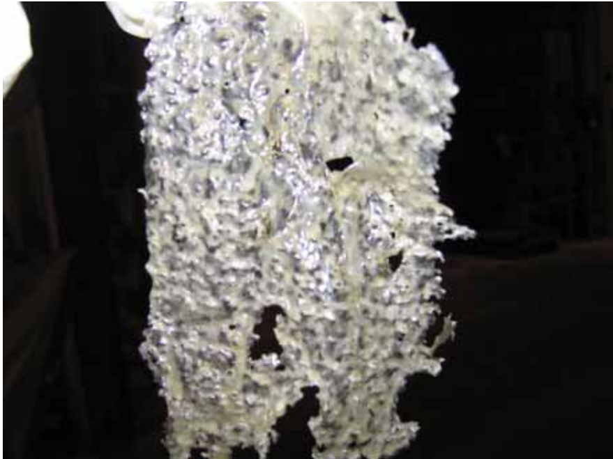
Figure 2 - DECON 188 removed from textured surface
