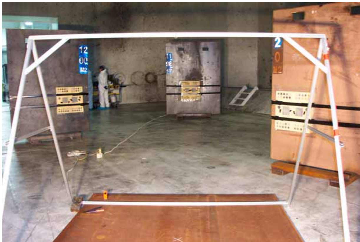
Figure 2. Placement of sample holder on steel blast shields inside the confined firing facility. The aluminum from in photo was used to suspend mock RDD 1 m above the floor.
