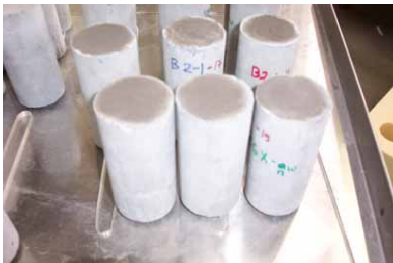
Figure 1. Examples of concrete cores placed in CFF chamber.
