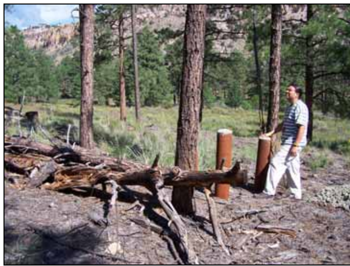
Fig. 6. Markers were set at the Bayo Canyon, New Mexico, Site to inform the public of an excavation restriction imposed because of Sr-90 residuals in soil.
