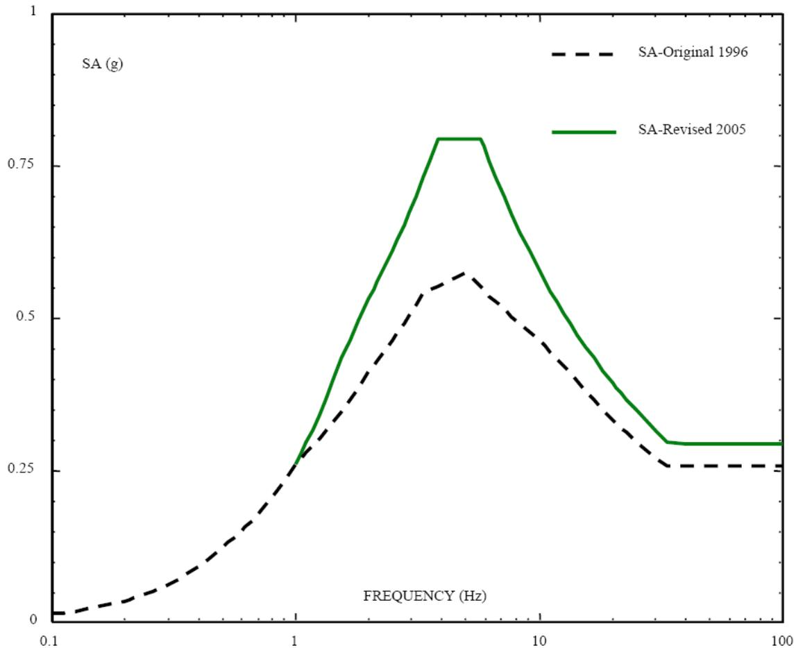
Fig. 3. Original 1996 and revised 2005 horizontal design spectra at 5% damping [2]
