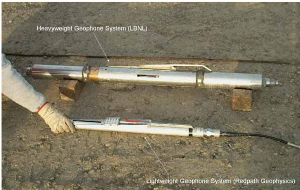
Fig. 7. Geophone systems used for downhole seismic logging
