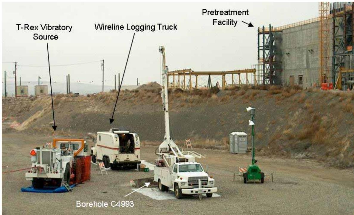
Fig. 6. Downhole seismic logging of borehole C4993 with vibratory source.
