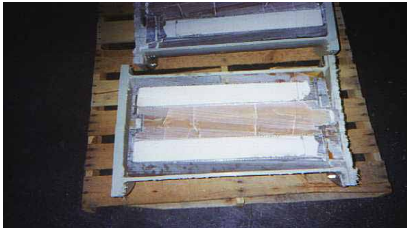
Fig. 3 Solidified package cut in half to show full impregnation of UOP-911 media.
