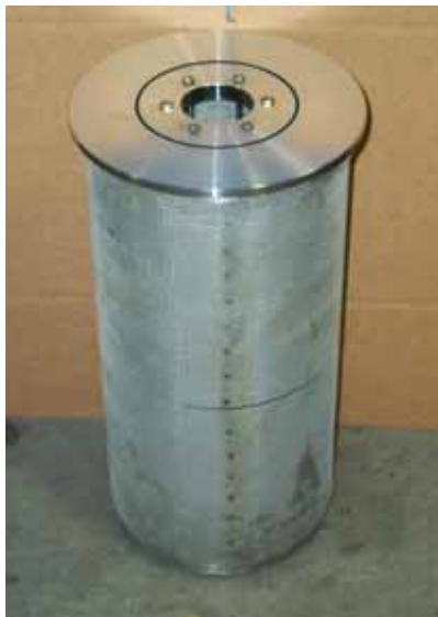
Fig. 1. Filter Canister with a 7.5–10 cm (3”-4”) inner annulus filled with UOP-911 media.
