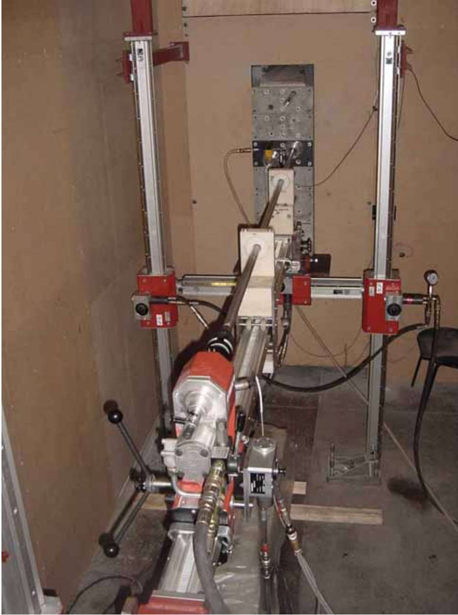
Fig. 4. Drilling Rig inside inactive mock up of the induction room
