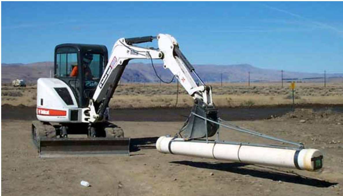
Fig. 4. Multiple array gamma detector for locating irradiated fuel fragment.
